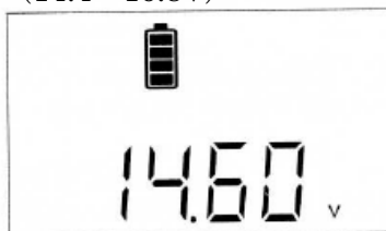
Fig 18. Battery overvoltage setting
