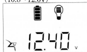
Fig 19. Battery low-voltage return value setting
